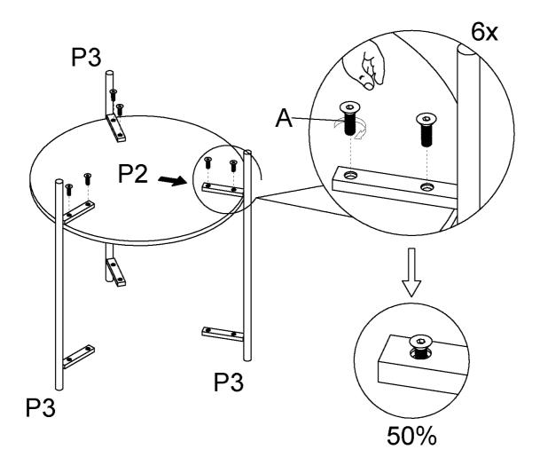
NOTE: ONLY TIGHTEN SCREWS 50% UNTIL ALL SCREWS ARE IN PLACE
