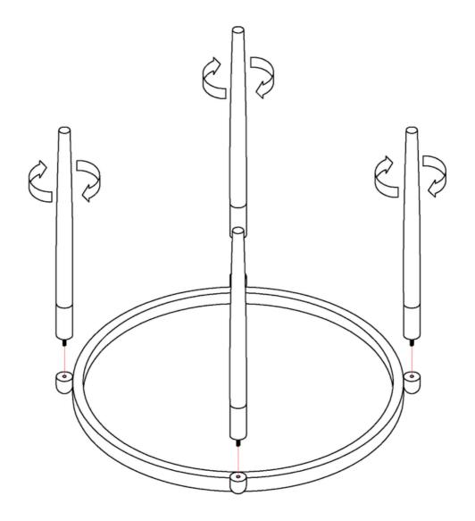
PLACE THE FRAME (PART 1) SECURELY ON THE FLOOR. SCREW THE X4 LEGS (PART 2) INTO THE FRAME (PART 1)
