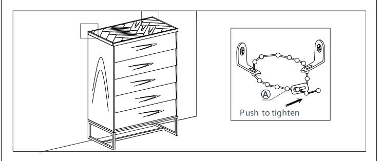
FINAL Step: Attach anti tilt strap or bracket to wall WARNING:
