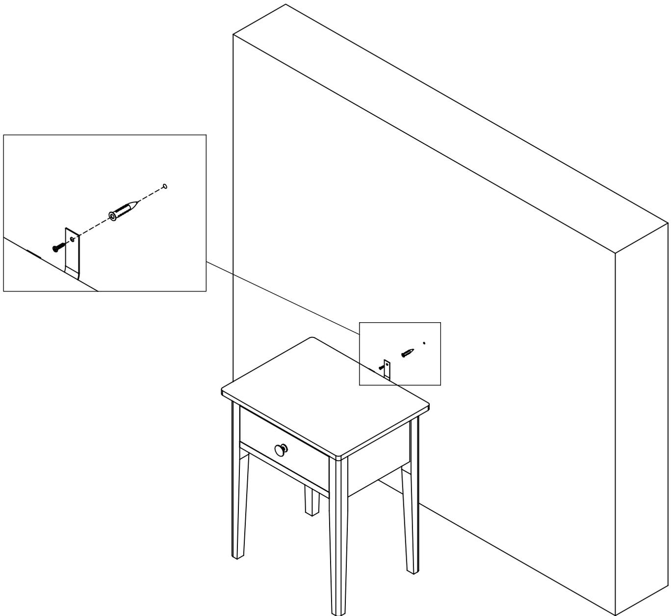
FINAL Step: Attach anti tilt strap or bracket to wall
