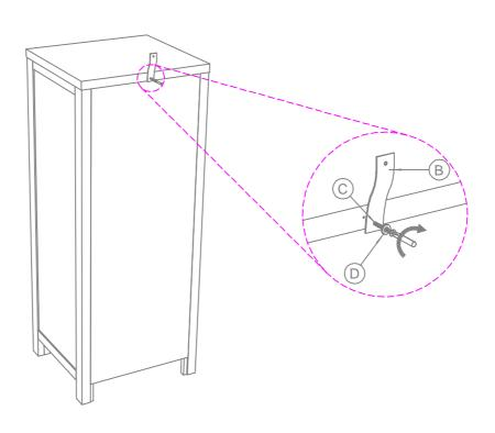
Make two holes with diameter 8mm on the wall, The hardware supplied is suitable for concrete, plaster or wood wall. For other wall types, please see your local hardware store.
