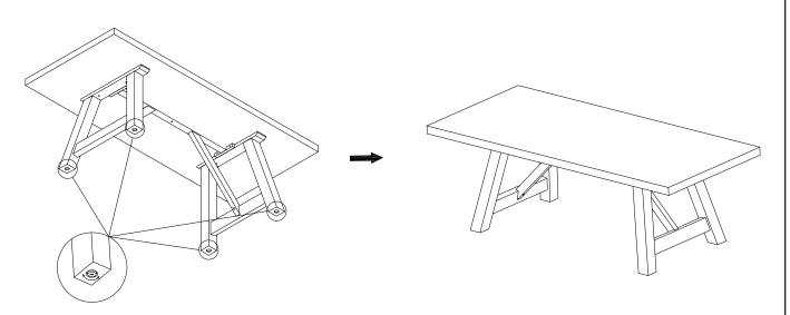
Ensure that all bolts are completely tightened
