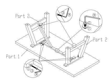
Ensure that all bolts are completely tightened
