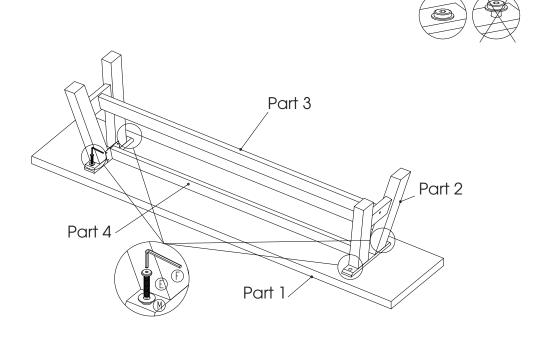
Ensure that all bolts are completely tightened
