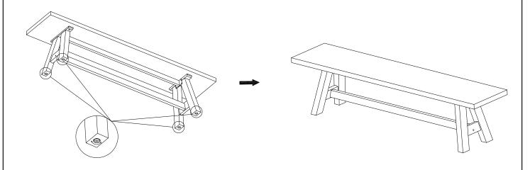
Ensure that all bolts are completely tightened
