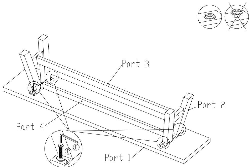
Ensure that all bolts are completely tightened
