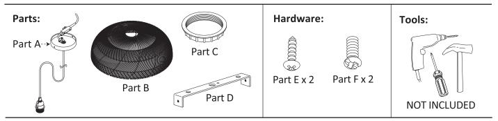
This fitting must be installed by a qualified electrician in accordance with the latest AS/NZS 3000 and relevant amendments
