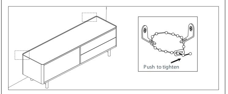
FINAL Step: Attach anti tilt strap or bracket to wall WARNING:
