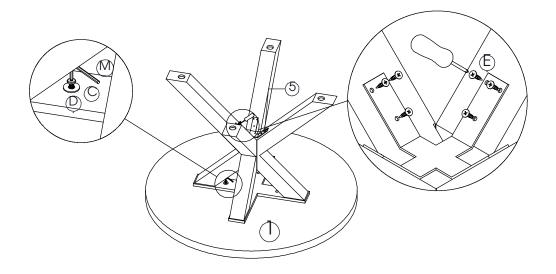
Ensure that all bolts are completely tightened
