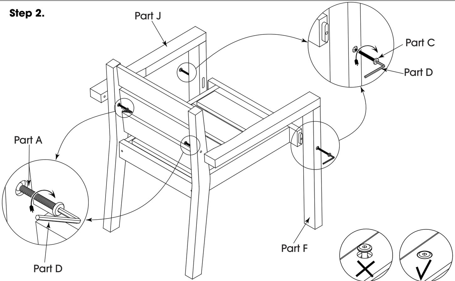
“Ensure that all bolts are completely tightened”
