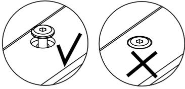
“Do not completely tighten Bolts”
