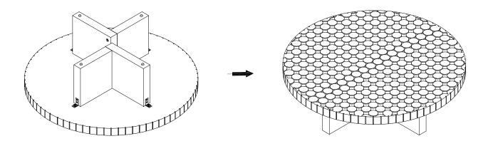
Ensure that all bolts are completely tightened
