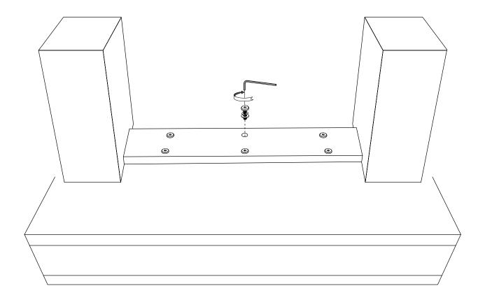
**Step 4:** Place the desk upright ensuring to evenly apply pressure to each leg. Uneven pressure can lead to damage.
