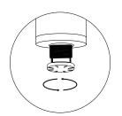
use adjusters at base of the feet if ground in uneven.
